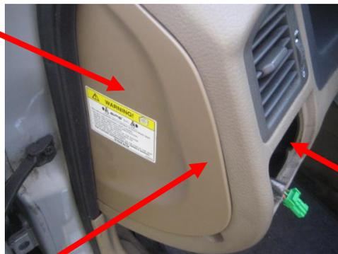
Inside you can feel some small plastic lockers on the top which you press down and at the same time press the panel out in the top from behind. Disconnect the cable in the back.
