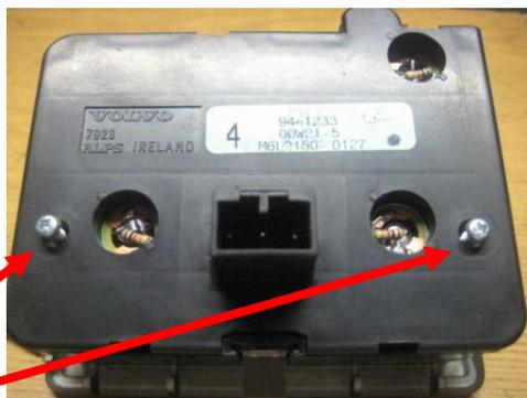
Loosen the 2 screws in the back of the panel.
